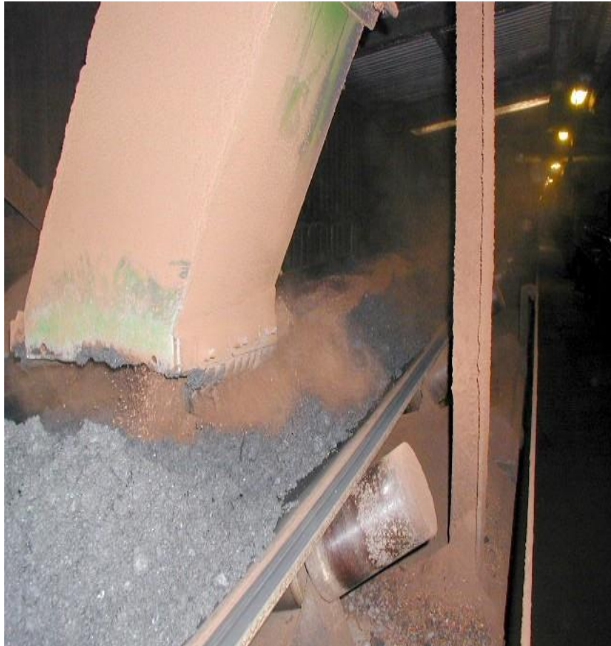
Figure 3.2 Granular olive residue material being dropped on top of coal on the main coal conveyor at a large coal power plant.
