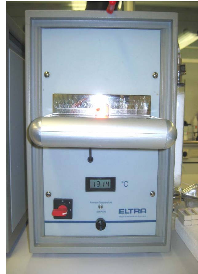
Analyzer for S, C According to method prEN 15289
