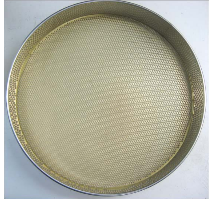
3,15 mm sieve according to ISO 3310 Particle size distribution prEN 15149
