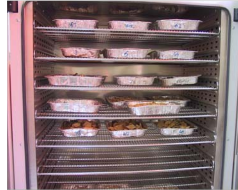
Drying oven, moisture content prEN 14774-1 – 3
