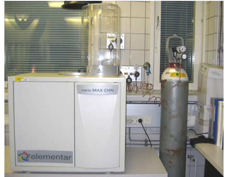
CHN-analyzer According to method prEN 15104
