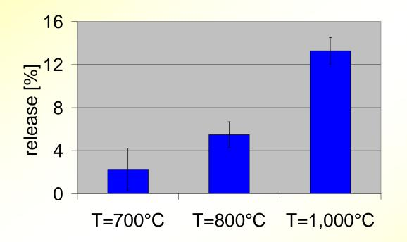
Release of K from the fuel to the gas phase during pellet charcoal combustion; results from test runs at a lab-scale reactor
