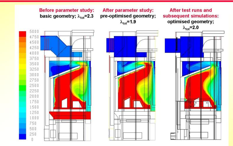
Iso-surfaces of CO concentrations [ppmv] in the flue gas in the vertical symmetry plane of the stove
