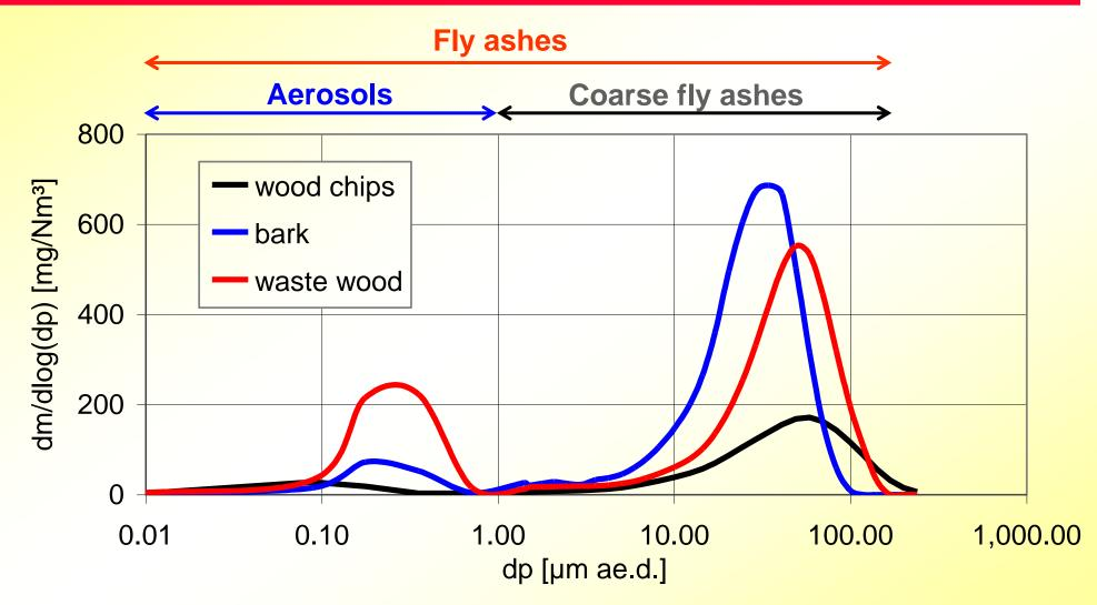
Data related to dry flue gas and 13 vol.% O<sub>2</sub>; results from grate-fired combustion systems
