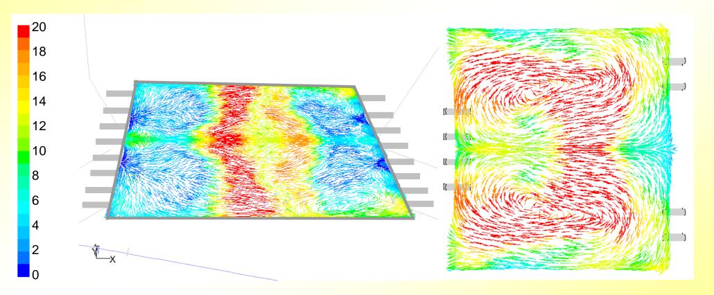
Flue gas velocity vectors [m/s] in a horizontal cross-section directly above the secondary air nozzles; simulations for full load operation
