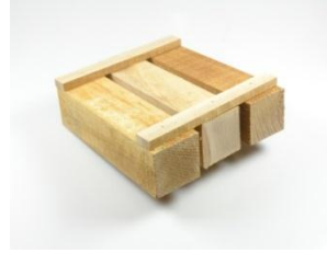
standard test fuel used : 7x7 cm beech wood
