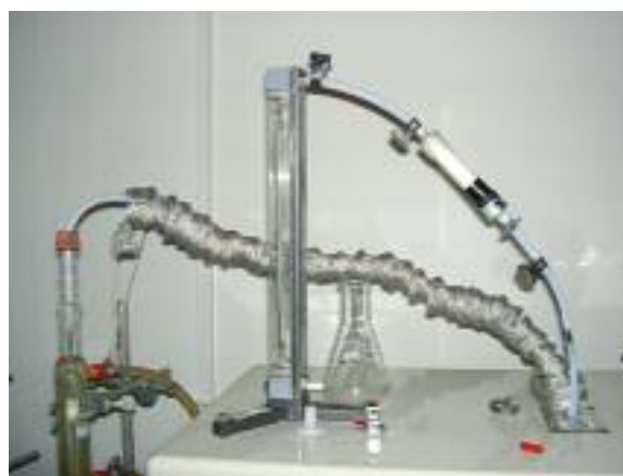
Fig 10. The flow meter, the water trap and the cotamination trap together with the heating mantle.
