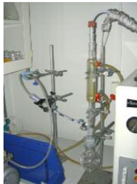
Fig 12. The collection system with cooler, glass flask, carbon tubes and water trap.
