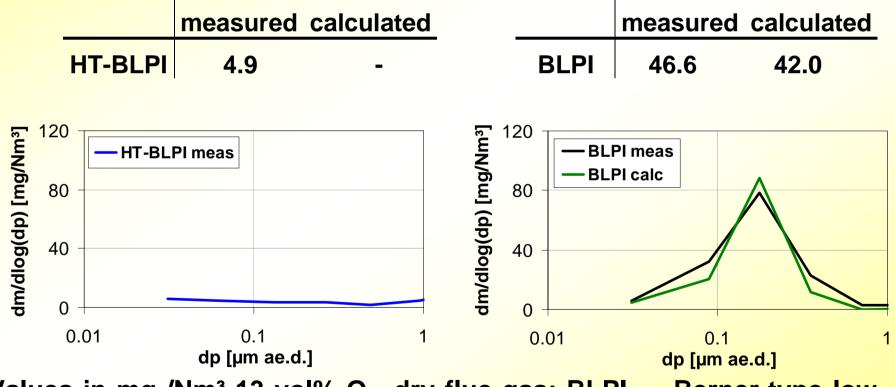
Values in mg /Nm<sup>3</sup> 13 vol% O<sub>2</sub>, dry flue gas; BLPI ... Berner-type low pressure impactor; HT-BLPI ... high temperature BLPI; ae.d. ... aerodynamic diameter
