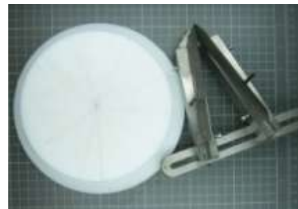
stamping plate with special knife
