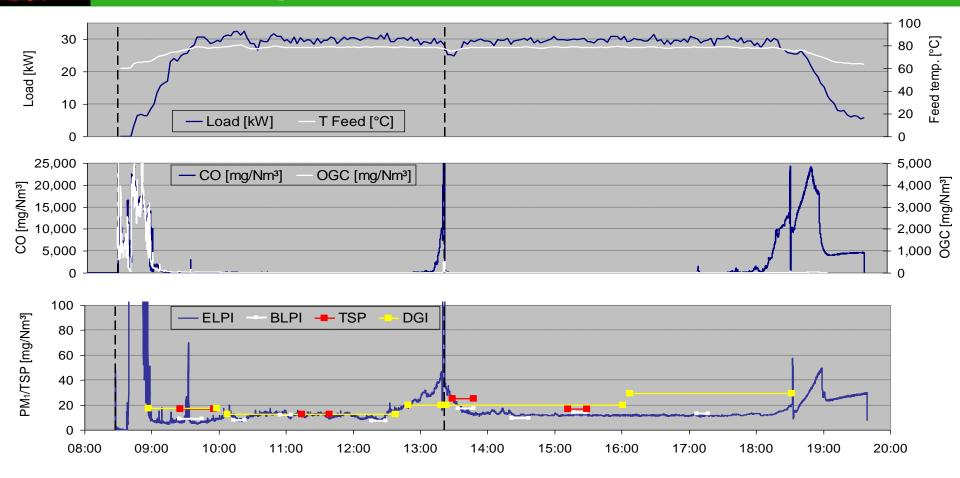
Explanations: fuel: logwood according to ÖNORM M 7132; data related to dry flue gas and 13 vol% O<sub>2</sub>; T Feed ... feed temperature; load ... boiler load; the BLPI, TSP and DGI lines indicate the measured PM concentration over the respective sampling period
