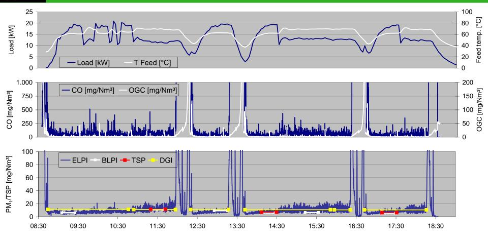
Explanations: fuel: pellets according to ÖNORM M 7135; data related to dry flue gas and 13 vol% O<sub>2</sub>; T Feed ... feed temperature; load ... boiler load; the BLPI, TSP and DGI lines indicate the measured PM concentration over the respective sampling period Slide 11
