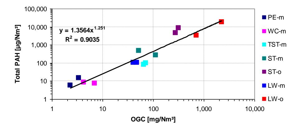
Explanations: PE-m ... modern pellet boiler; WC-m ... modern wood chip boiler; LW-m ... modern logwood boiler; LW-o ... old logwood boiler; ST-m ... modern stove; ST-o ... old stove; TST-m ... modern tiled stove; statistical evaluation: trend p<0.1
