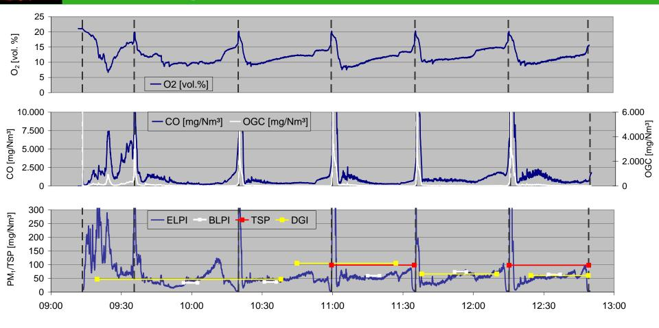
Explanations: fuel: logwood according to ÖNORM M 7132; data related to dry flue gas and 13 vol% O<sub>2</sub>; the BLPI, TSP and DGI lines indicate the measured PM concentration over the respective sampling period
