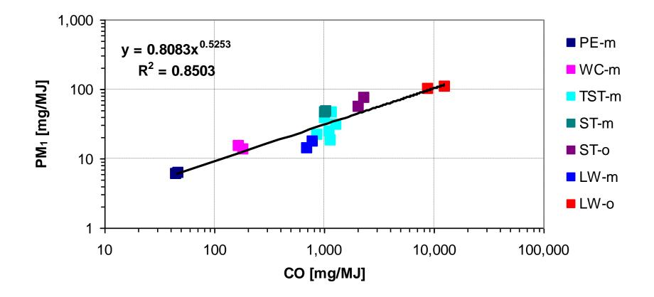
Explanations: mean values over the test runs performed; PE-m ... modern pellet boiler; WC-m ... modern wood chip boiler; LW-m ... modern logwood boiler; LW-o ... old logwood boiler; ST-m ... modern stove; ST-o ... old stove; TST-m ... modern tiled stove; statistical evaluation: significance p<0.05
