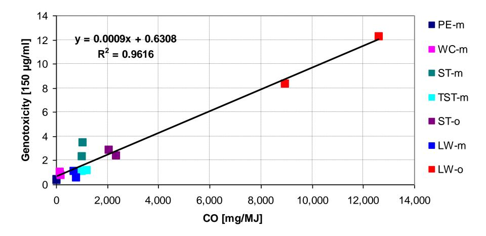
Explanations: PE-m ... modern pellet boiler; WC-m ... modern wood chip boiler; LW-m ... modern logwood boiler; LW-o ... old logwood boiler; ST-m ... modern stove; ST-o ... old stove; TST-m ... modern tiled stove; statistical evaluation: significance p<0.05
