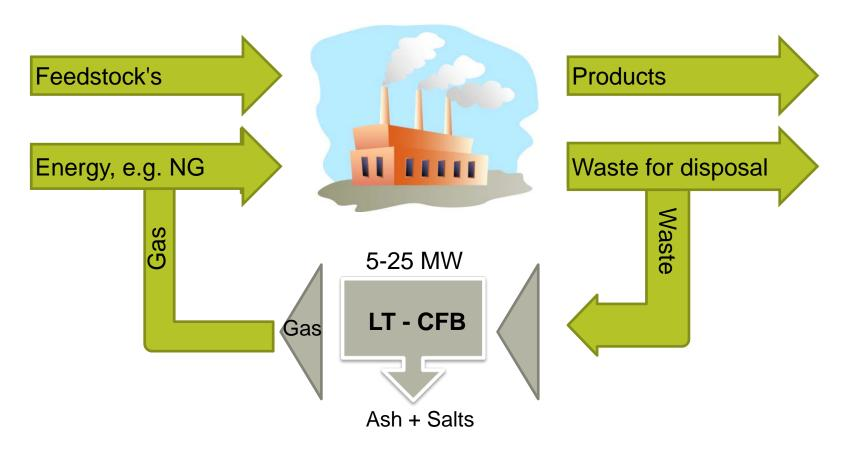
The LT-CFB gasifier can use cheap local waste fractions to replace expensive natural gas
