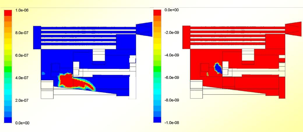
Iso-surfaces of the reaction rates [kmol/(m<sup>3</sup>\*s)] of the reaction N + NO  $\rightarrow$  N<sub>2</sub> + O for the reduction to N<sub>2</sub> (left) and of the reaction N + NO  $\leftarrow$  N<sub>2</sub> + O for the formation of NO from N<sub>2</sub> (right) in the symmetry plane of the combustion chamber and the boiler
