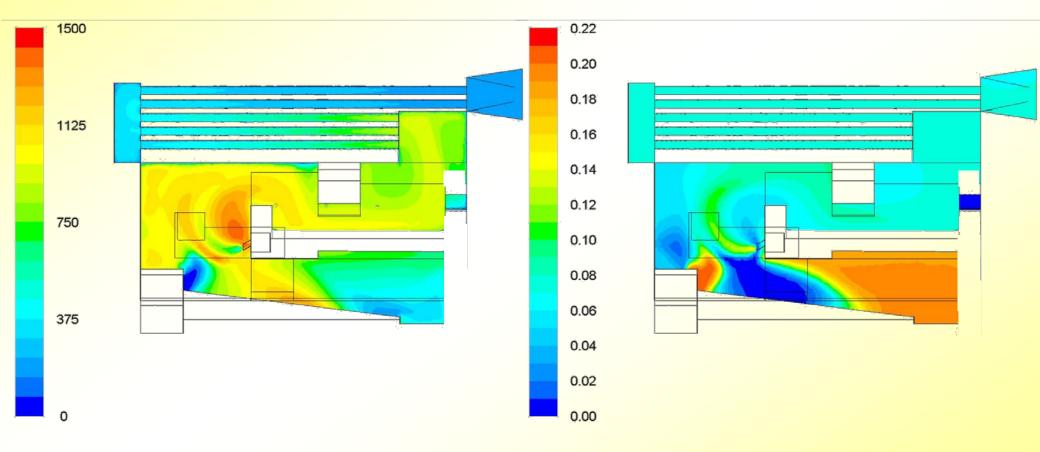
Iso-surfaces of temperatures [°C] (left) and  $O_2$  concentrations [m<sup>3</sup>  $O_2$ / m<sup>3</sup> wet flue gas] (right) in the symmetry plane of the combustion chamber and the boiler
