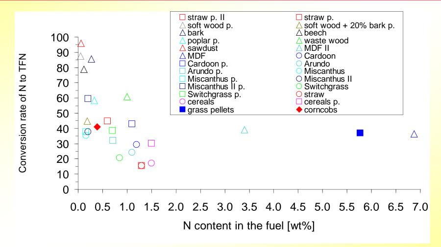
explanation: all data taken from reactor experiments with lab-scale pot furnace; TFN ... mass of all N-moles contained in NO, NH<sub>3</sub>, NO<sub>2</sub>, HCN und N<sub>2</sub>O, released from the fuel bed
