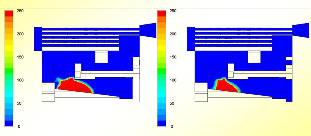
Iso-surfaces of NH<sub>3</sub> concentrations [ppmv w.b.] (left) and HCN concentrations [ppmv w.b.] (right) in the symmetry plane of the combustion chamber and the boiler
