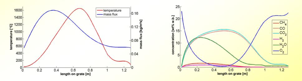
Calculated profiles of temperature, mass flux and species concentration in the flue gas along the grate for grass pellets
