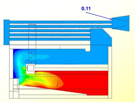
Iso-surfaces of local TFN/TFN<sub>in</sub> ratios in the symmetry plane of the combustion chamber and the boiler <u>explanation</u>: TFN ... mass of all N-moles contained in NO, NH<sub>3</sub>, NO<sub>2</sub>, HCN und N<sub>2</sub>O, released from the fuel bed
