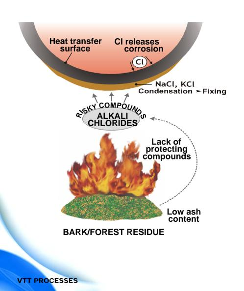
Direct connection to fouling and corrosion risk of the boiler
