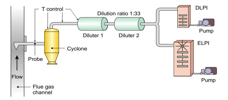
Particle mass size distribution by DLPI (Dekati Low Pressure Impactor) Particle number size distribution by ELPI (Electrical Low Pressure Impactor)
