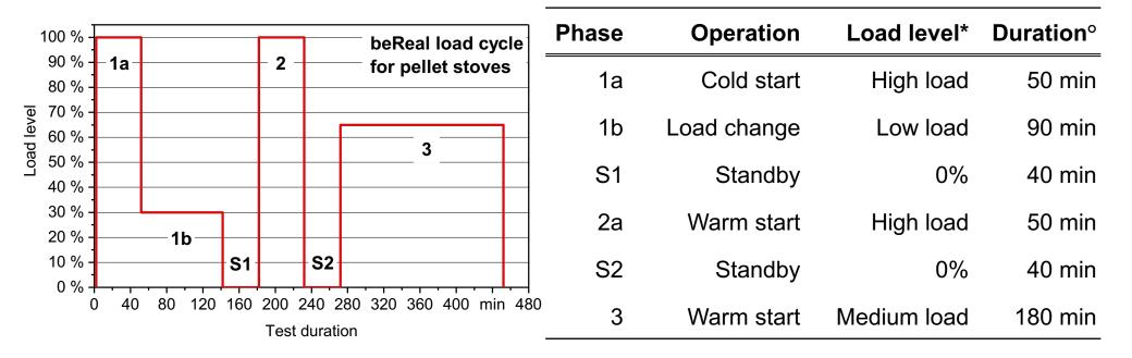
• **Duration:** The recording of measurement parameters is launched when starting stove operation (i.e. when pushing the start button for ignition).
