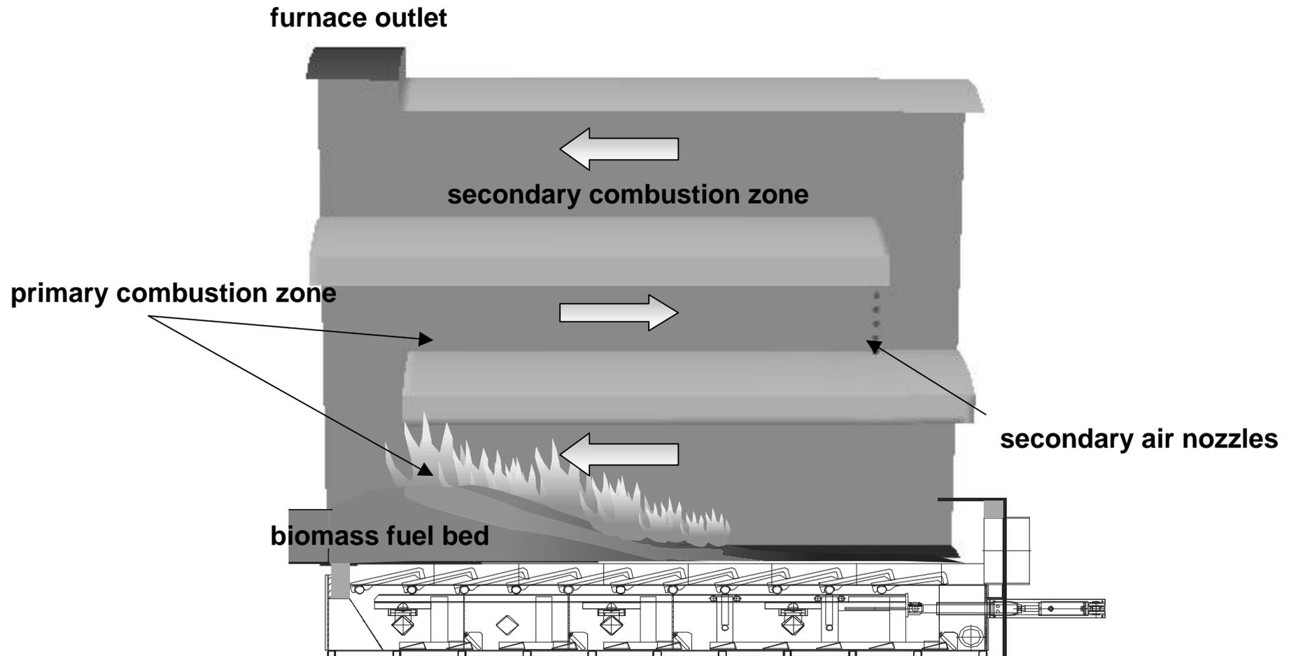
**Pilot-scale Low-NO<sub>x</sub> furnace (440 kW<sub>th</sub>)
