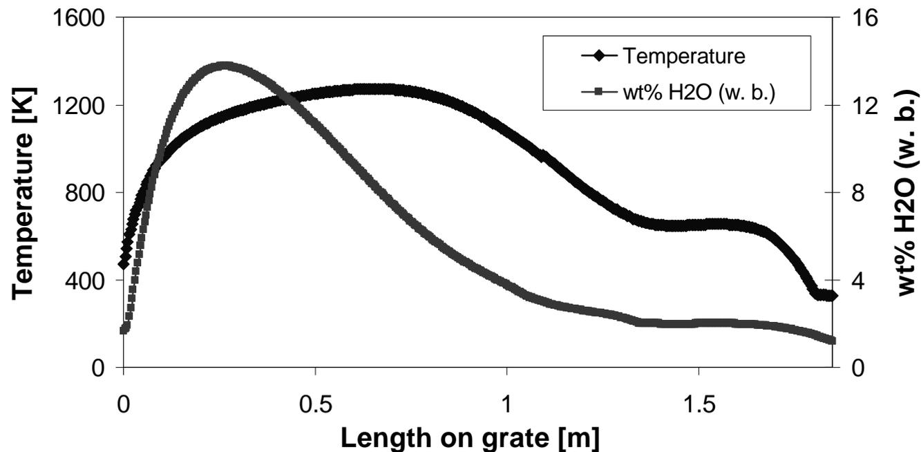
Profiles of temperature and  $\text{H}_2\text{O}$  concentration of the flue gas along the grate
