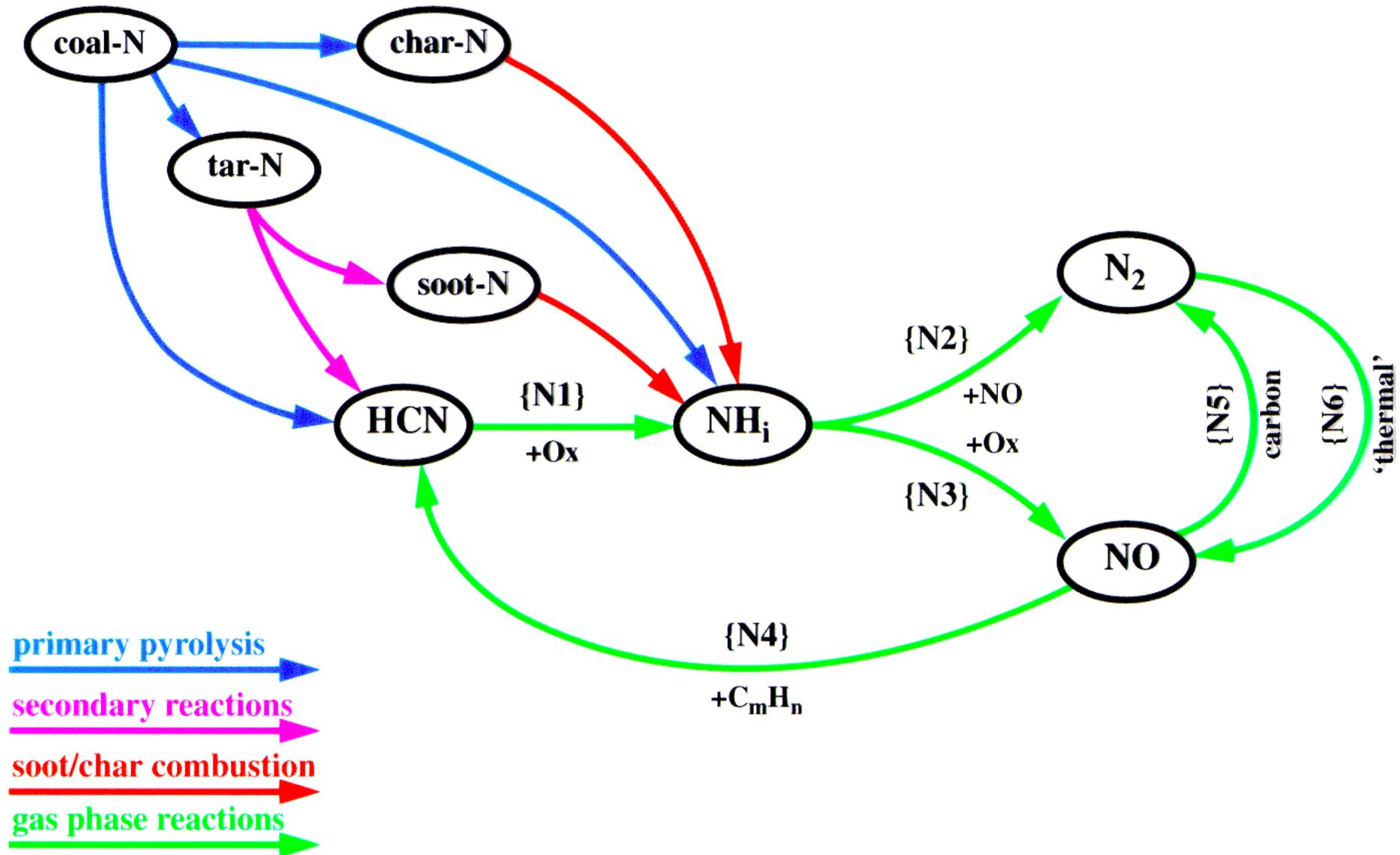
Kinetic Reaction Scheme of Fuel-Nitrogen Conversions
