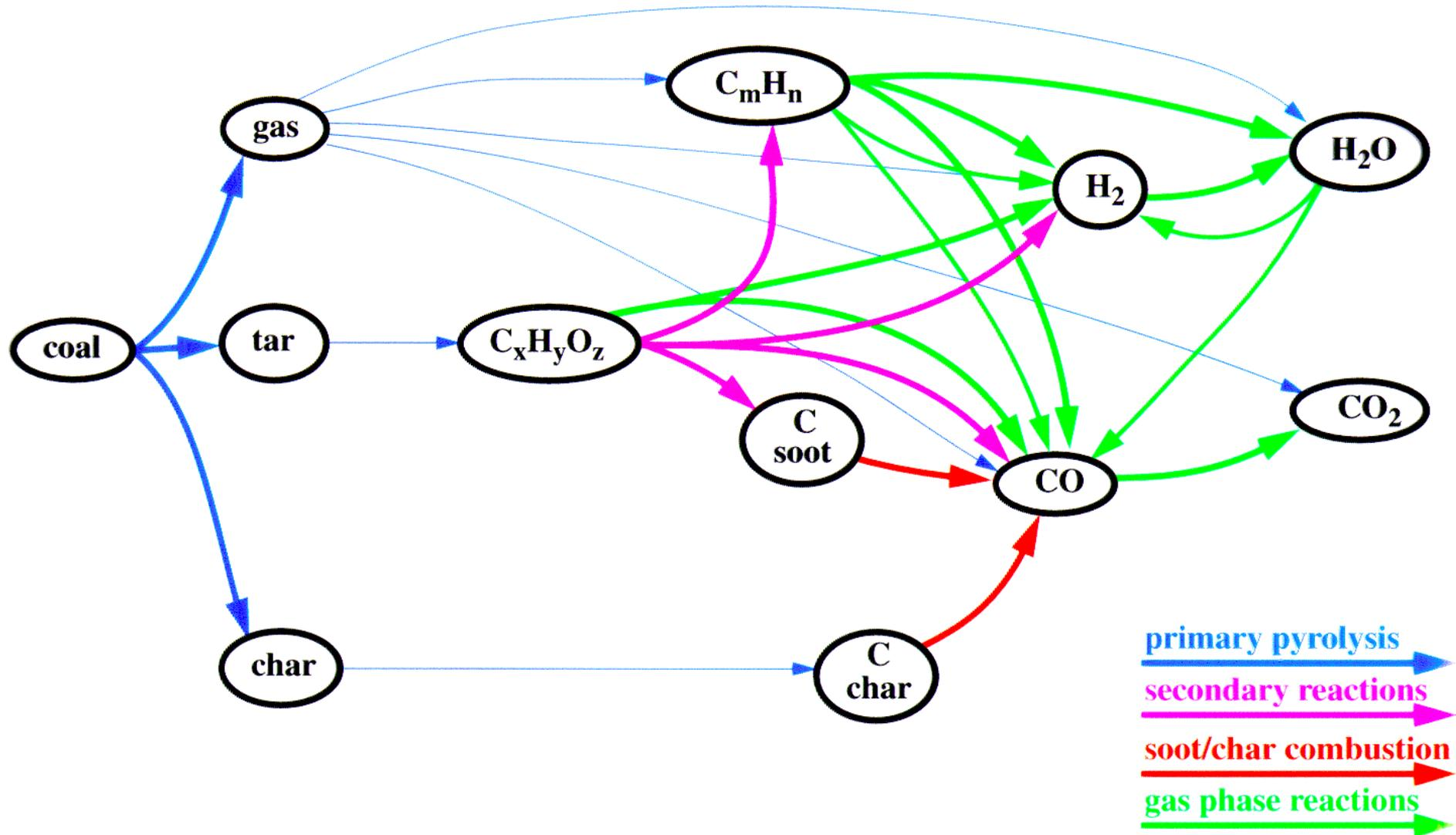
Extended Kinetic Reaction Scheme of Pulverized Coal Combustion
