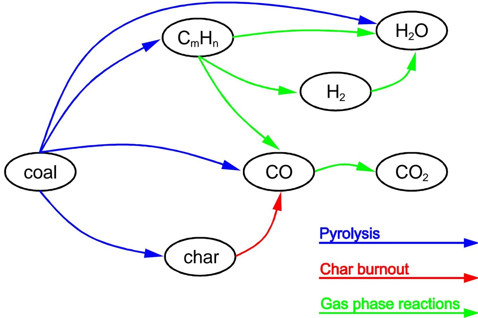
Reaction Scheme of Coal Combustion
