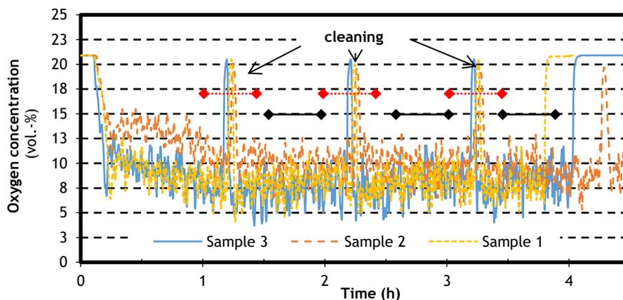
*Figure 9: Approach for experimental evaluation regarding the impact of the cleaning interval on emission and efficiency performance of pellet stoves (red: average oxygen content during 30 minutes interval with cleaning and black: average oxygen content during 30 minutes interval without cleaning)*
