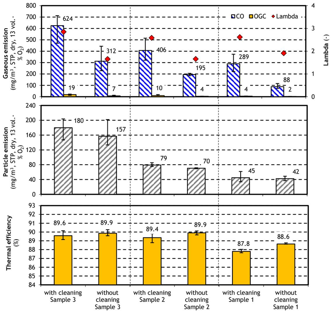
Figure 10: Results of experimental evaluation regarding the impact of the cleaning interval on emission and efficiency performance of pellet stoves
