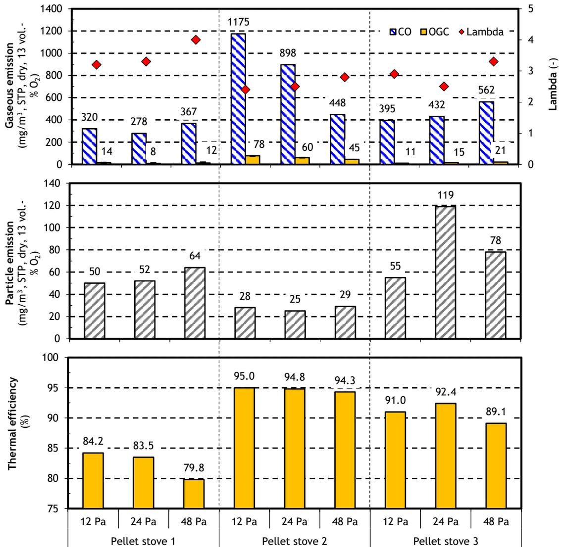
Figure 8: Results of experimental evaluation regarding the impact of draft conditions on emission and efficiency performance of pellet stoves
