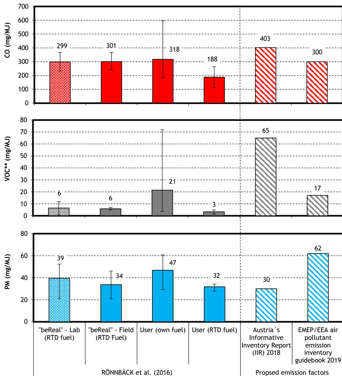
Figure 14: Comparison of lab and field test results of beReal project (same EN 14785 pellet stoves) with proposed emission factors (EFs). Error bars represent the minimum and maximum values determined. \*\* VOC emission factors based on proposed NMVOC-EF, assuming 40% methane of total VOC emissions (see Equation 2)
