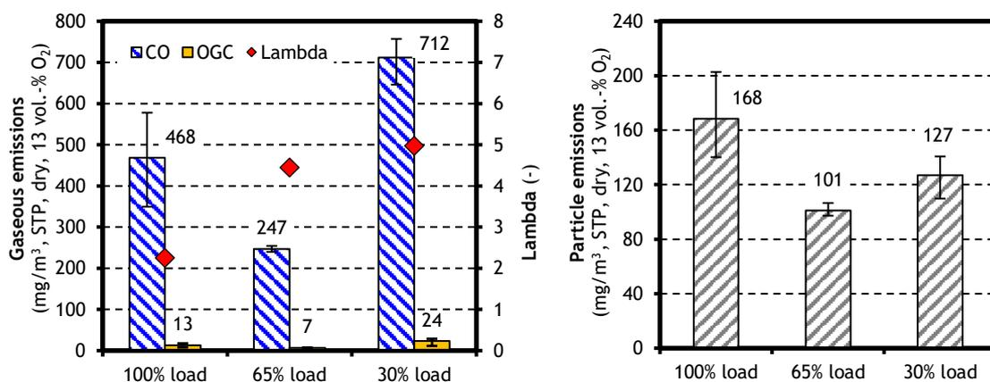
**Figure 7: Influence of load settings on gaseous and PM emissions (n=3, error bars represent the minimum and maximum measurements)**
