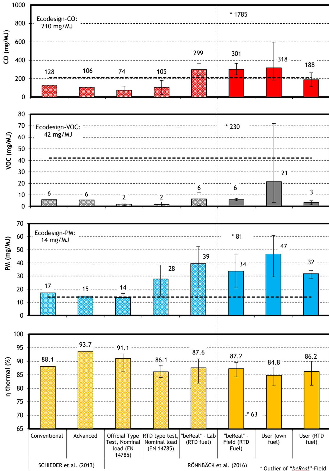
Figure 13: Comparison of official type test (ott) results with lab and field test results. Error bars represent the minimum and maximum values determined. The dashed black lines represent the ELVs of future ecodesign requirements for pellet stoves [23].
