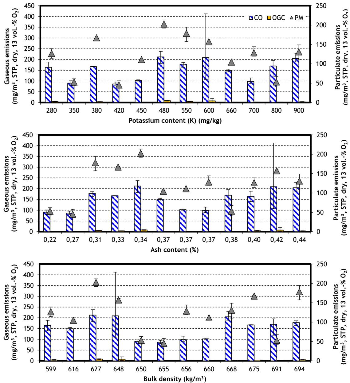
Figure 5: Emission concentrations of 12 different EN<sub>plus</sub> certified pellet samples in relation to potassium content (top), ash content (middle) and bulk density (bottom) used in the same pellet stove in consecutive tests
