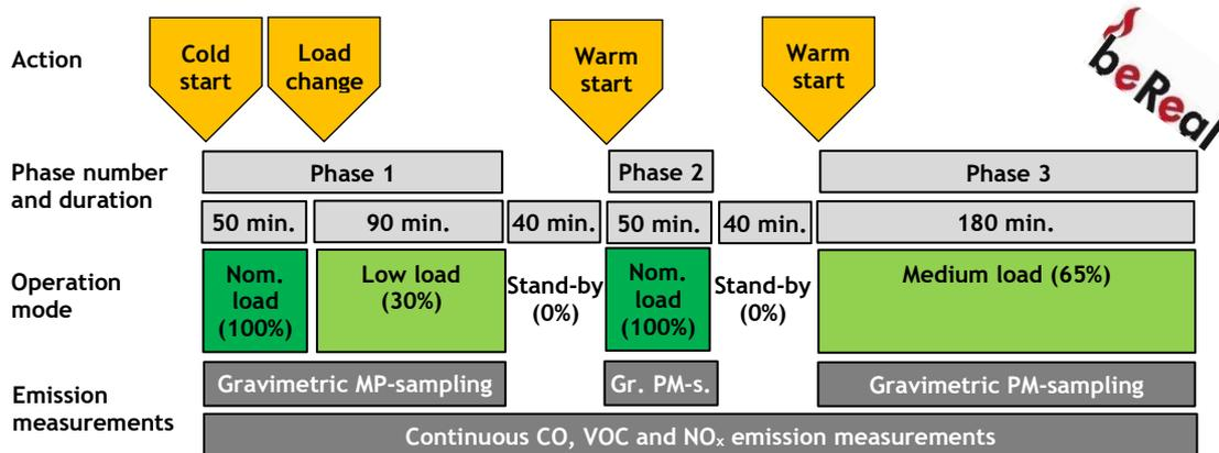
Figure 11: Scheme of “beReal” test concept for pellet stoves (without water jacket)
