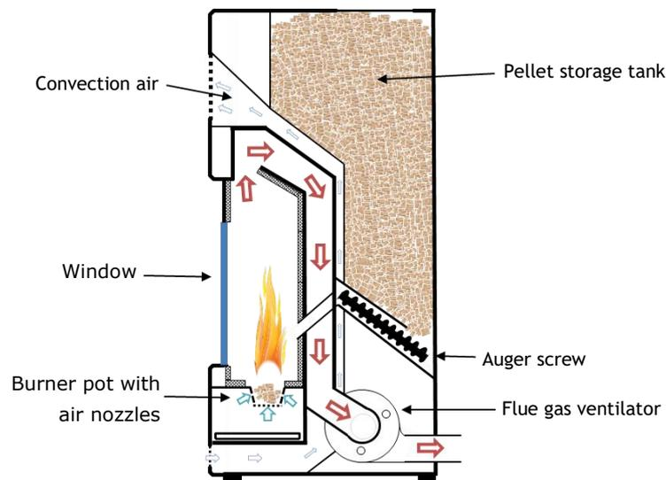
*Figure 1: Scheme and main features of a pellet stove*
