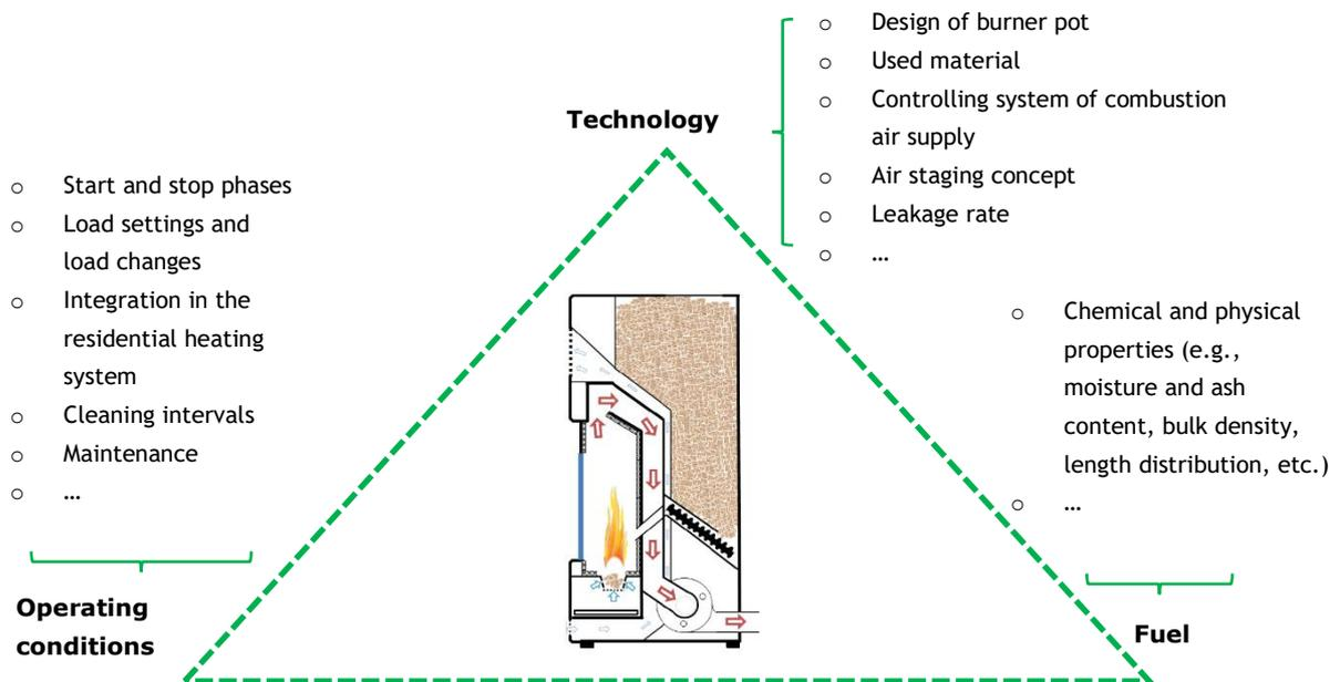
Figure 3: Main aspects that could influence the real-life performance of pellet stoves regarding emissions and thermal efficiency
