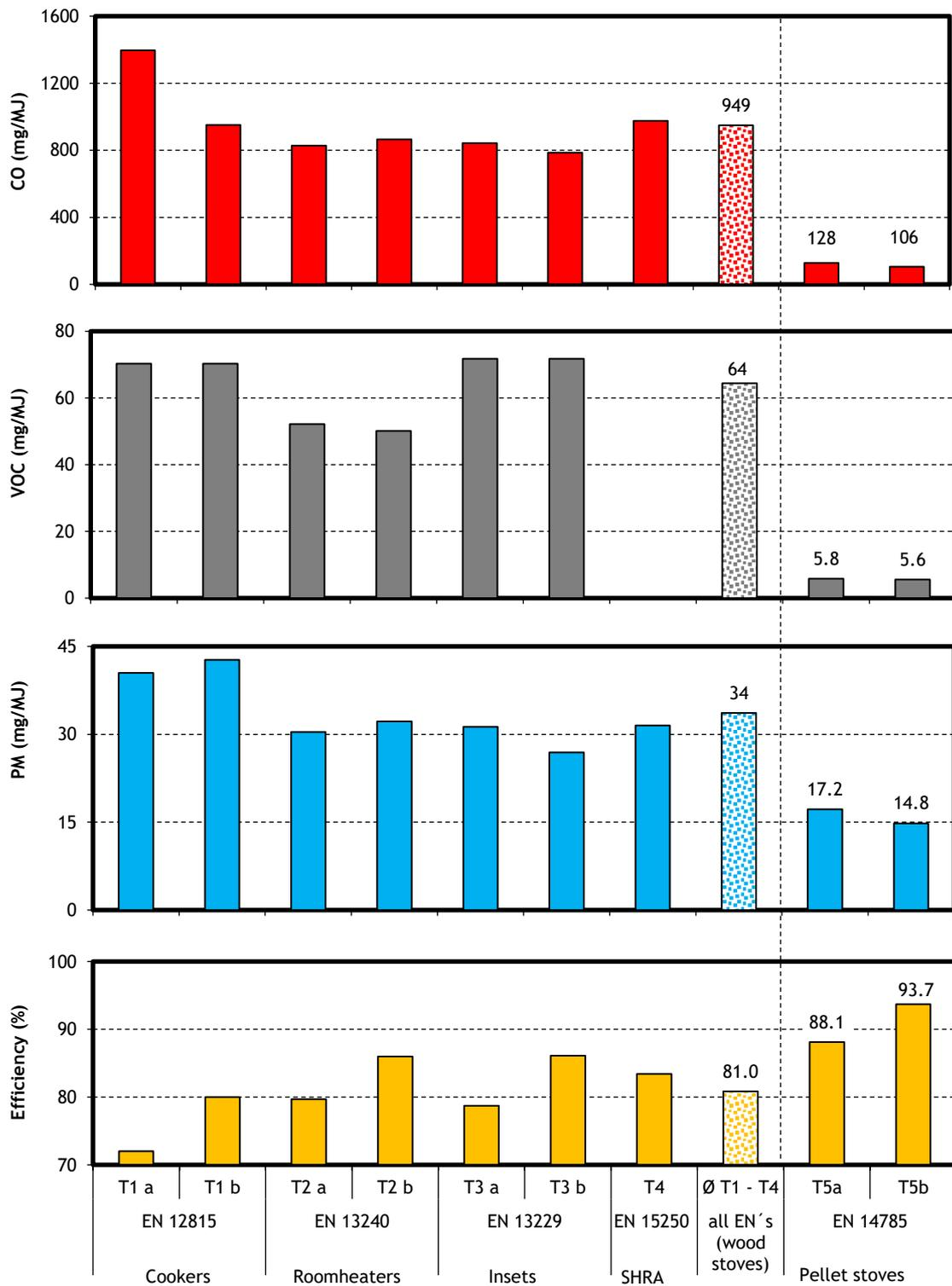
Figure 12: Overview of official type test (ott) results for different types of firewood as well as pellet stoves (conventional technologies...a / modern technologies...b).
