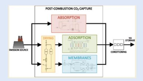
Taken from Zarco et.al. 2021 ..... Postcombustion CO2 Capture: A Comparative Techno-Economic Assessment of Three Technologies Using a Solvent, an Adsorbent, and a Membrane | ACS Engineering Au
